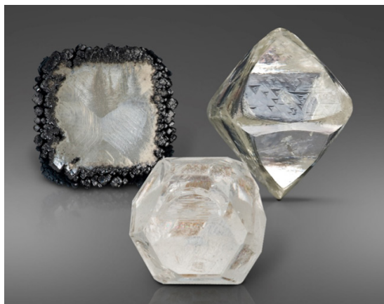
Laboratory-grown CVD rough diamond (left), laboratory-grown HPHT rough diamond (middle), and natural rough diamond (right). Composite image. This CVD diamond rough crystal weighs 6.37 ct and was grown at GIA’s laboratory in New Jersey. Photo by Robert Weldon/GIA.
