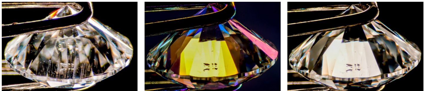
Extreme lack of strain observed in HPHT-grown diamond using diffused light (left), CPF and First-Order Red Compensator (middle), and Cross-Polarized Filters (right)
