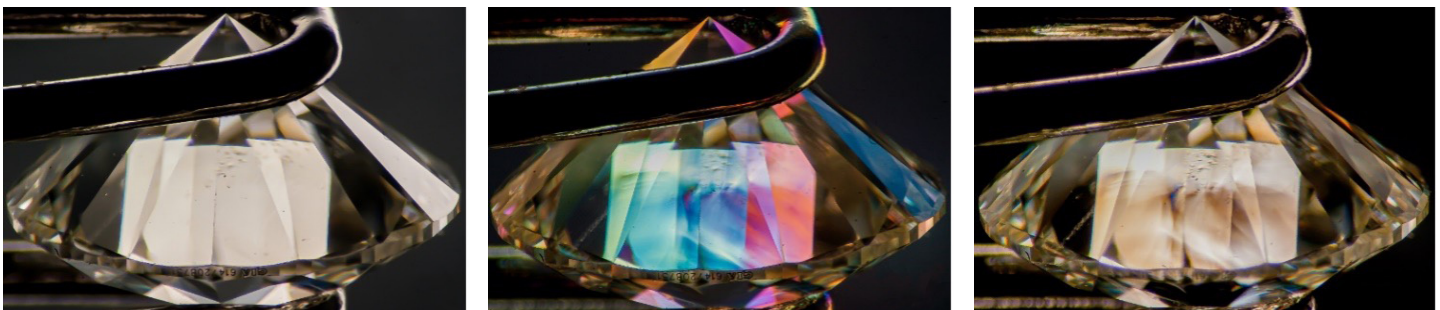
Typical smudgy, irregular strain observed in natural Type Ia(A/B) diamond using diffused light (left), CPF and First-Order Red Compensator (middle), and Cross-Polarized Filters (right)
