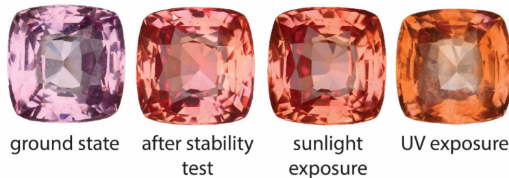
Figure 1: In some extreme cases, color-unstable sapphires can vary from a purplish pink color in the ground state to pure orange when exposed to UV light.
