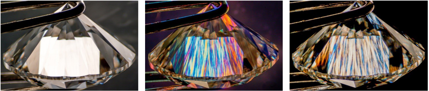
Parallel, columnar strain observed in CVD-grown Diamond using diffused light (left), CPF and First-Order Red Compensator (middle), and Cross-Polarized Filters (right)
